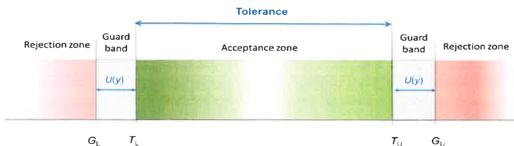
Figure 3: Display of acceptance and rejection zones for the normalized safe rejection interval
